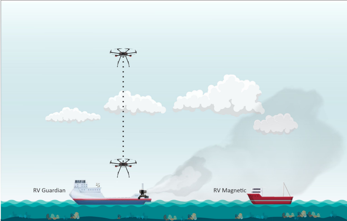
Figure 1: Positions of RV Guardian and RV Magnetic vessels during the Marine Cloud Brightening campaign on Jan-Feb 2022. SSA particles were released during the campaign on board the RV Guardian while CCN and aerosol, measurements were performed on board the RV Magnetic. The distance between the vessels was typically about 1.5 km. During spraying time, measurements of the atmospheric thermodynamic conditions (T, P, RH) above RV Guardian were performed by drones up to heights of \sim 1-2 km.
