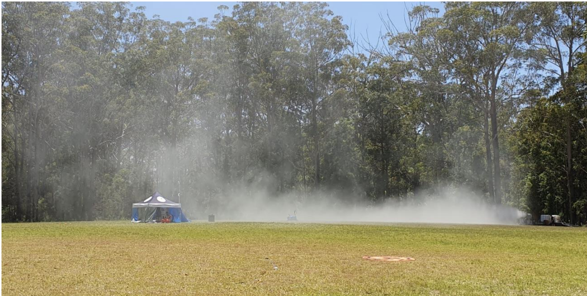
Figure 1., A sea water fog plume generated with the modified proof-of-concept fog cannon and measured with the aerosol instruments on the tower and tent, fifty metres away.
