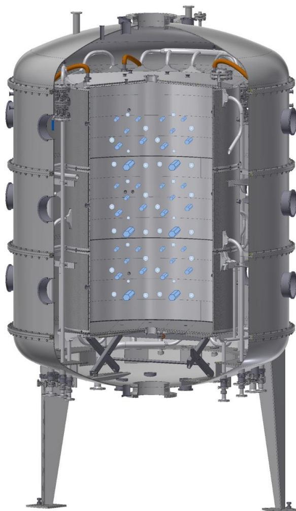
Figure 1. Construction of the AIDA vacuum and cloud chambers.
