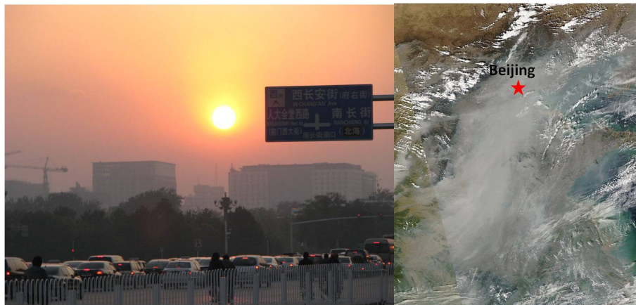
Figure 2: An example of a visual in situ (left) and satellite (right) observation on 13 th Oct. 2008. The photo has been taken in the city centre of Beijing, China, about an hour after the satellite overpass time. The satellite data is a RGB-composite image from the MODerate Imaging Spectroradiometer (MODIS) instrument onboard the Aqua satellite. In the satellite image the bright white areas are clouds while haze due to aerosols appears as different shades of gray.
