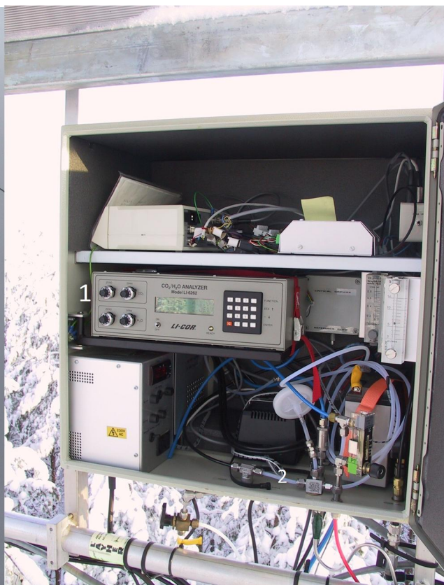
Figure 7. 1) LI-6262 CO 2 & H 2 O analyser 2) sample air/calibration gas switching valve
