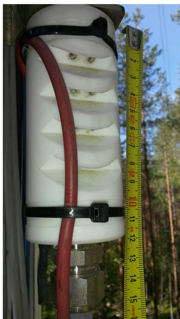
Figure 9. Sample air inlet in the high tower (photo courtesy of Janne Levula).
