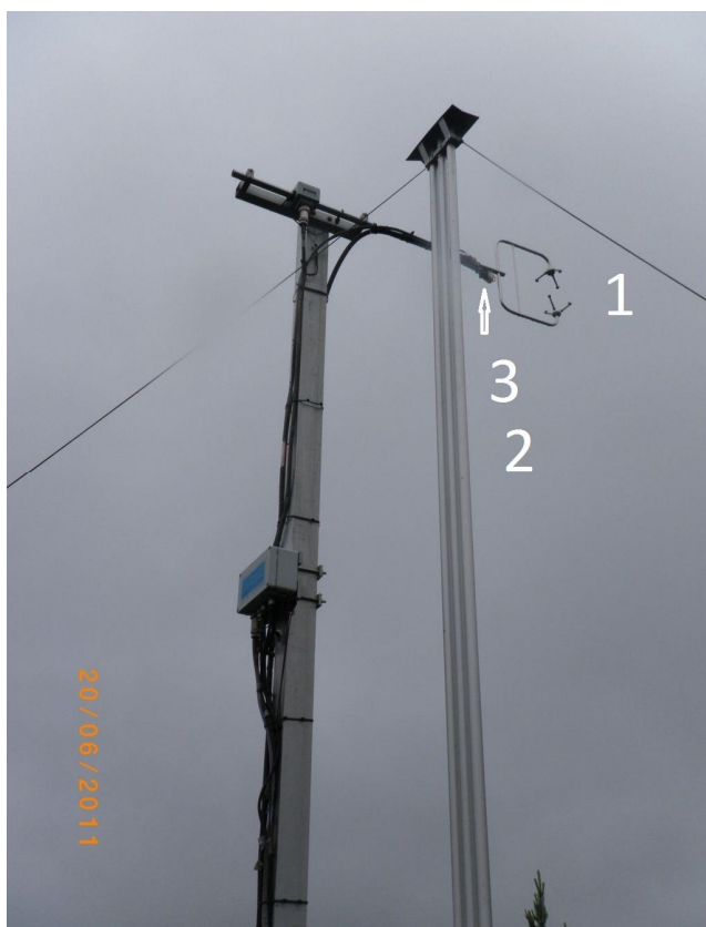
Figure 6. 1) Solent HS sonic anemometer; 2) sample lines of Relaxed Eddy accumulation; 3) sample air inlet.
