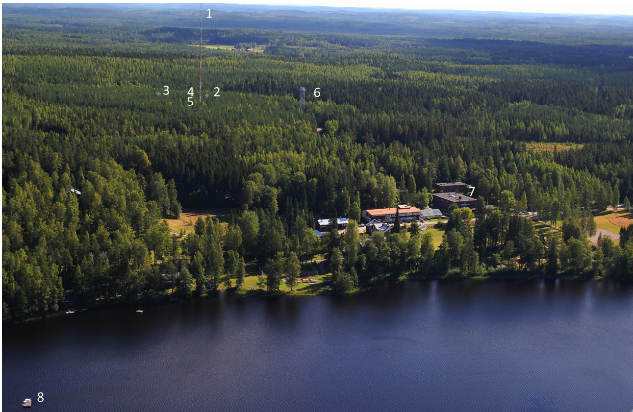
Figure 3. SMEAR II measurement site seen from the West over the lake Kuivajärvi. 1) 127 m high tower; 2) 18 m high scaffolding tower; 3) and 4) 16 m and 17 m scaffolding towers; 5) SMEAR cottage; 6) 35 m high tower; 7) Forestry field station; 8) floating platform. (Photo courtesy of Katri Leino).
